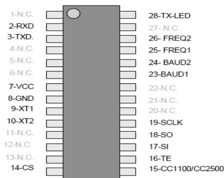
Figure 3. The diagram of RF Transceiver pin configuration
