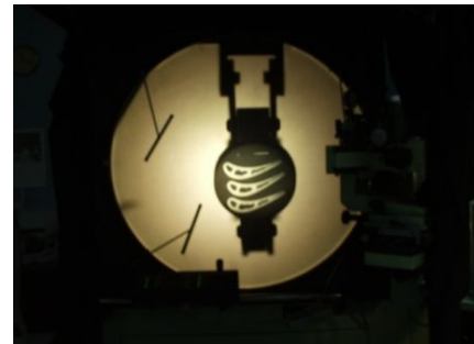
Fig. 5 : Inspection of cut-sections of turbine blade in optical profile projector
