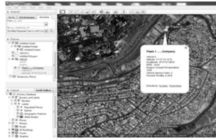
Figure 7. Google Earth Snapshot showing the live location and motor parameters of the robot
