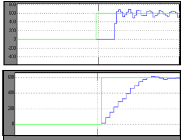
Figure 6. Comparison of Torque Response of IFOC and DTC Respectively
