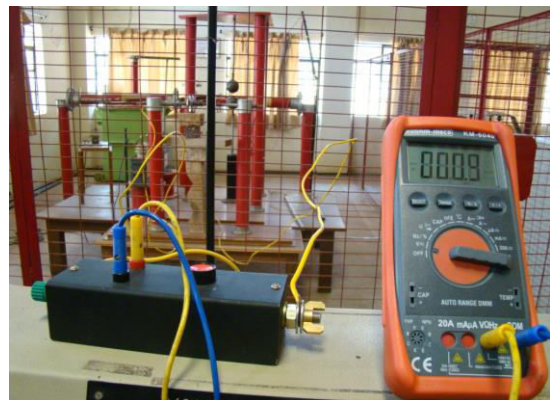
Figure 1: Experimental set-up for measurement of leakage current against the applied voltage.
