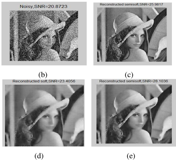
Fig. 3 (a) : The original Lena image (b) noisy image (c) Result of LBWDT (d) Result of LBWDAW (e) Result of the proposed method
