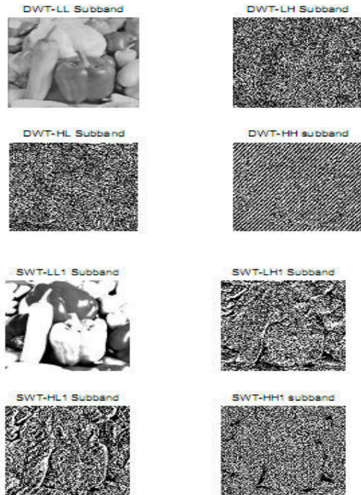
Fig.5. LL, LH, HL, and HH subbands obtained by using DWT and SWT.
