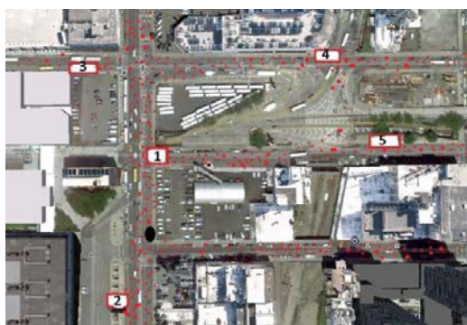
Fig. 8 (a) : Initial position of the robot and its particle distribution.
