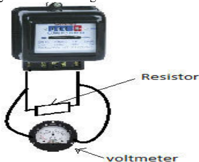
Figure 1 Circuit diagram of principle used in Smart Electrical Meters
