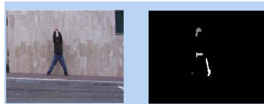
Figure 2. a) A frame from an aerobic sequence, b) The ROI obtained after background subtraction.
