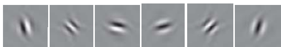
Fig 2 Two dimensional dual tree complex wavelets in spatial domain oriented at -75^\circ, -45^\circ, -15^\circ, 15^\circ, 45^\circ, 75^\circ respectively [10].
