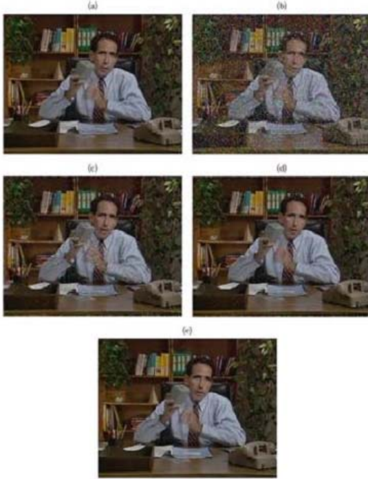
Fig. 2. The original 20th frame of the ‘‘Salesman’’ sequence (a), the frame corrupted by 20% random impulse noise (b) ( PSNR = 15.05 dB) and the result after the first (c) ( PSNR = 23.72 dB), second (d) ( PSNR = 29.42 dB) and refinement step (e) ( PSNR = 36.78 dB) respectively.
