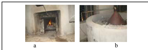
Figure 5. New furnace in operation: (a) Flaps covering entry point of combustion chamber, ash formed on combustion of firewood pulled out from underneath (b) rock insulation and piping from furnace fed to condenser for bamboo vinegar production.
