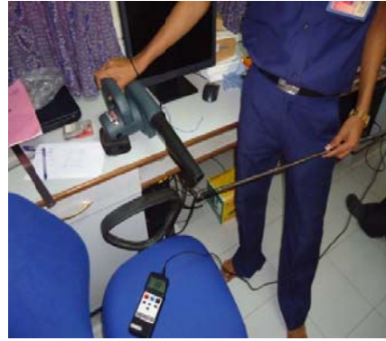
Fig 5- measurement of air velocity by hot wire anemometer
