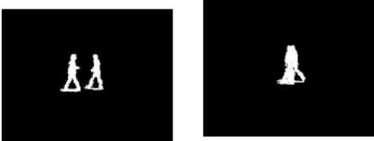
Fig 4 :Two objects in the previous frame merged into single object in frame2.
