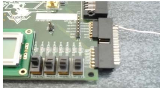
Figure 14. The slide switches and the connector which makes the junction between the pulse generator and the board.
