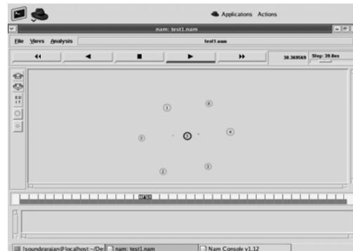
Fig. 3.1 A snapshot showing the route 0-5-4 is selected by DSR
