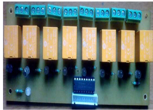
Fig. 1.3 : Relay Panel Board
