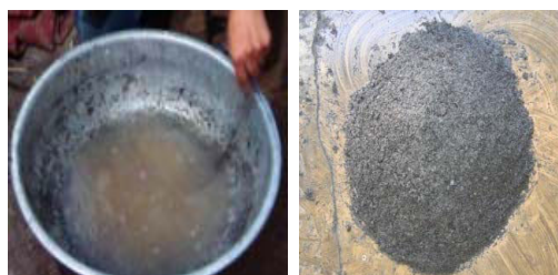
Fig. 2: Binder preparation and carbonized charcoal mixed with the binder
