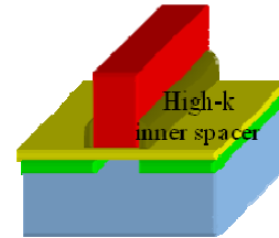
Fig. 2 : Corner technology based device showing mono layer technology (inner layer)
