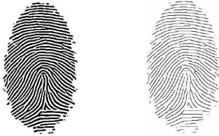
Fig.4 Binarized and thinned fingerprint image
